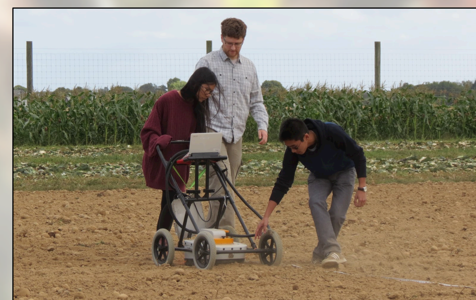
Honor students Claudia Yan and Edwin Cho collect data across a potato field using the Common Offset method. The GPR is located in the enclosure at the bottom of the cart and the information is collected by a computer. Photo Credit: Clyde Thomson
