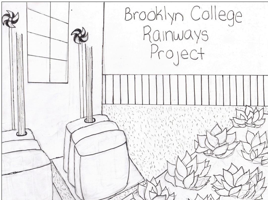
Original concept art of the gutter/drainage system on the sidewall of Whitehead Hall. As water falls, it turns the pinwheels on the building's wall, which in turn spins the motors at our charging station. The water then collects in the rain tanks at the base of the wall and is stored for use in the rain garden.
